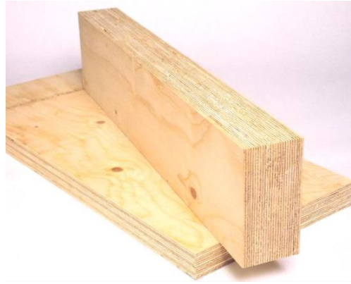
Figura 2.13 - Laminated Veneer Lumber – LVL
